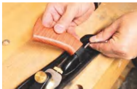
▲ You can pivot the rear tote to gain a better position when doing bevel work
